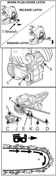
Note: Align the brake connector of the Bar/Clutch Cover (C) to the groove on the side of the brake lever (Front hand guard).
