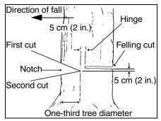
cut about 5 cm (2 in.) will act as a hinge when the tree falls, guiding it in the desired direction. When the tree starts to fall, kill the engine, place the saw on the ground and make your retreat quickly.
