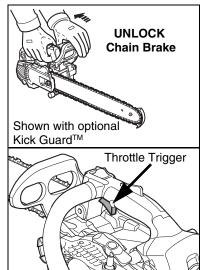
7. Be sure that saw chain stops moving when throttle trigger is released.
