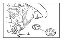
If the Oil Filter (a) is dirty, wash it in gasoline or replace it as follows: 2.
